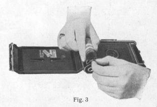
ber, as shewn in Fig. 3, and insert the film spool drawing out the flanges slightly until the pivots catch in the holes in each end of the spool. See that the word "Top" on the red protective paper comes on the side opposite to the winding-key. Then remove the adhesive strip which encircles the spool, draw the protective paper over both rollers and thread it into the longer slot in the empty spool in the other film chamber. (Fig. 4.)
